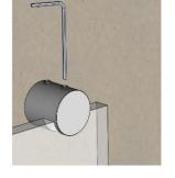
4 Slide the grips/panel onto the anchors. Tighten the outside M4 set screw once all grips are seated flush against the anchors.
