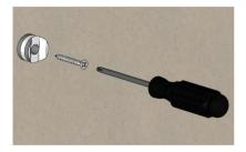
3 Install edge grips on the panels. Tighten the M4 set screw located inside the edge grip, after aligning the panels inside the edge grips.
